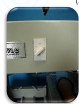
4. If you do not need to heat pieces installed on the sole rack (5) flip down the toggle switch (3). Only 4 lamps will stay on.
