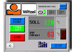
process it can also be controlled by an external temperature sensor (standard scope of delivery). For that just a thin wire sensor is placed at the edge of the Pre-Preg material, between the layers and plugged into the front panel of the control unit. Thus the entire heating process is controlled by the exact core temperature of the material.
