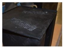
**Note:** You are sure that the charcoal is well packed inside the filter when you can't see the light passing throught the metal container.
