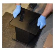
5. It is very important to fill completely the canister up to the edge. You can use yours fingers to push the charchoal each sides of the openings. Replace the black door with the two screws.
